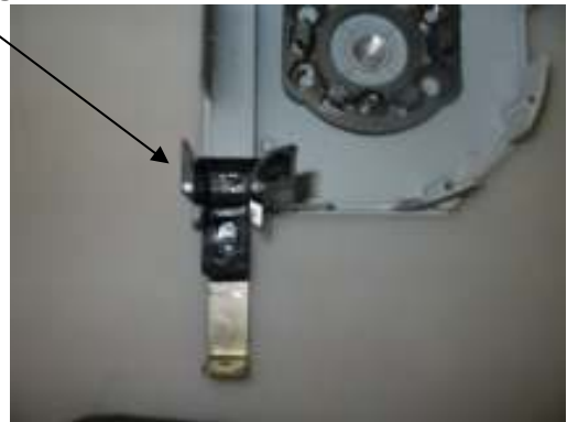
flat edge of entry guide towards rear, curved edge towards front of end cap
