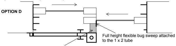
1 x 2 rectangular aluminum tube is self supported at the top and bottom with angle clips, the tube is not attached to the patio door panel
