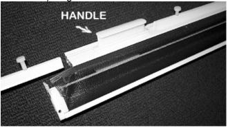
Step 6) Carefully replace the plastic end cap, threading the spline on the screen mesh into the cap as shown. Replace the screws from step 2. Be certain that the pan-head screw in the cap is backed off ½ turn after tightening. The cap must "float" in position.
